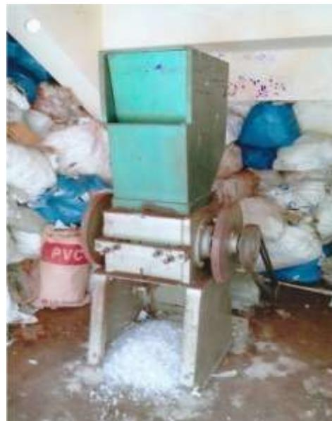
Plastic shredding machine installed at Balussery GP
