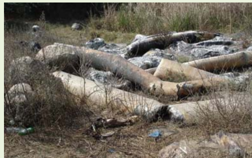
Burnt GRP pipes at the site relating to Part-IB works
