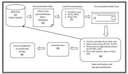
and activation of the chip. The diagram of the above process is shown in the following chart.
