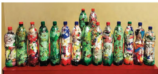
PET bottles filled with multi-layered plastic waste by children, to be converted into eco-bricks
