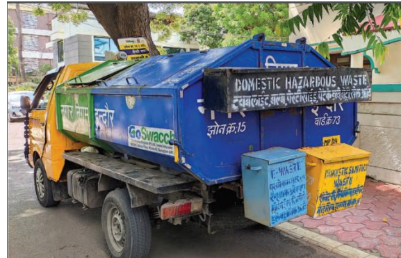
Figure 23 Compartmentalized vehicle for collection of biodegradables, non-biodegradable, domestic hazardous, electronic and sanitary wastes (Niti Aayog, CSE, 2021)
