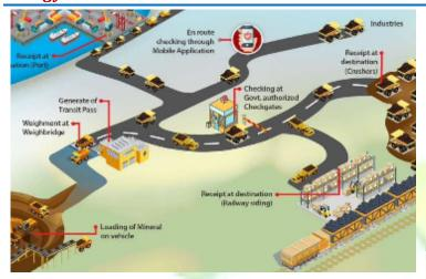
The diagram depicts the modalities of exploitation of underground minerals. their processing and further transportation to the industries for consumption, usage sites, ports and railway sidings for export/transportation across the States. The control mechanism and responsibility centers on mining operations and data
