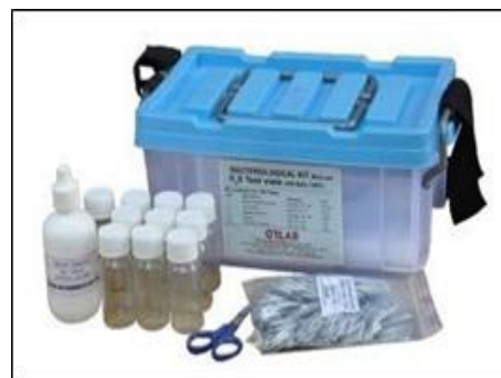
Photo 5.2: FTK for water
