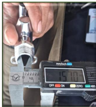
Photo 3.2: Picture showing 15mm taps being used in FHTC
