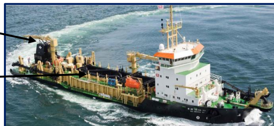
Figure 7.2 – Trailer Suction Hopper Dredgers (TSHD)
