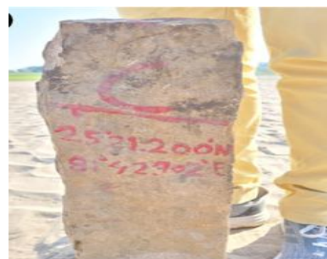
Figure:2.10- The only one permanent Pillar at Aman Brick Field at Bara found 80 meter away from its actual location
