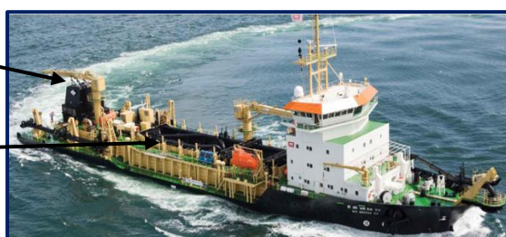
Figure 7.2 – Trailer Suction Hopper Dredgers (TSHD)
