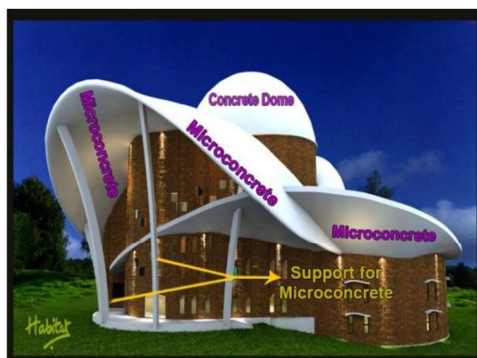
Figure 4.1: Architectural design of Space Theatre with cap brims fixed with micro concrete, prepared by Habitat Technology Group
