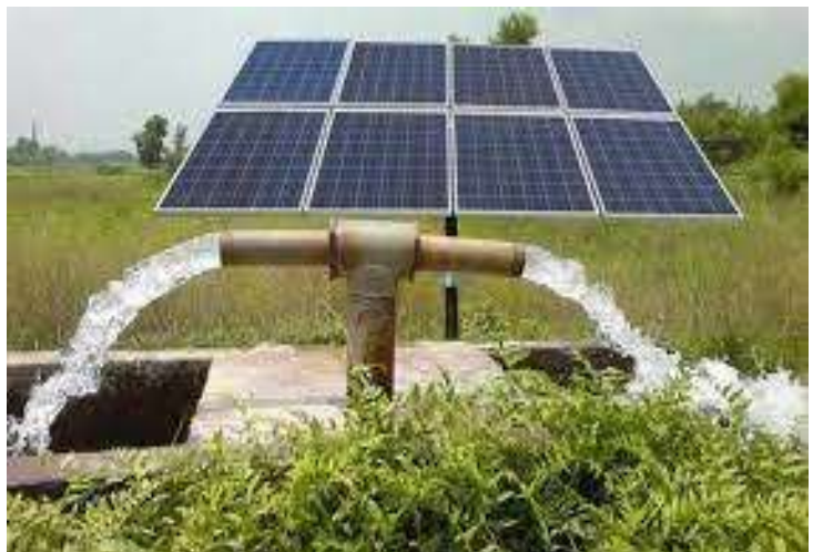
Picture No. 3.1: Solar Water Pump.
