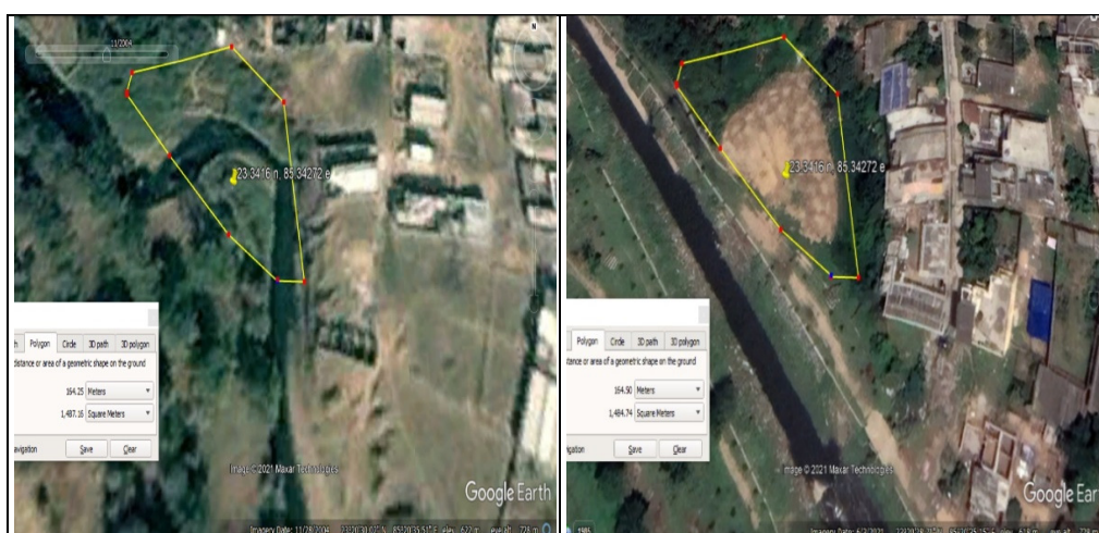
Picture 4.15: Satellite images of the river (Geographical co-ordinates: 23.3416 north and 85.34272 east), showing emergence of land (approximately 1487 metre sq), due to mechanical straightening of the meandering portion
