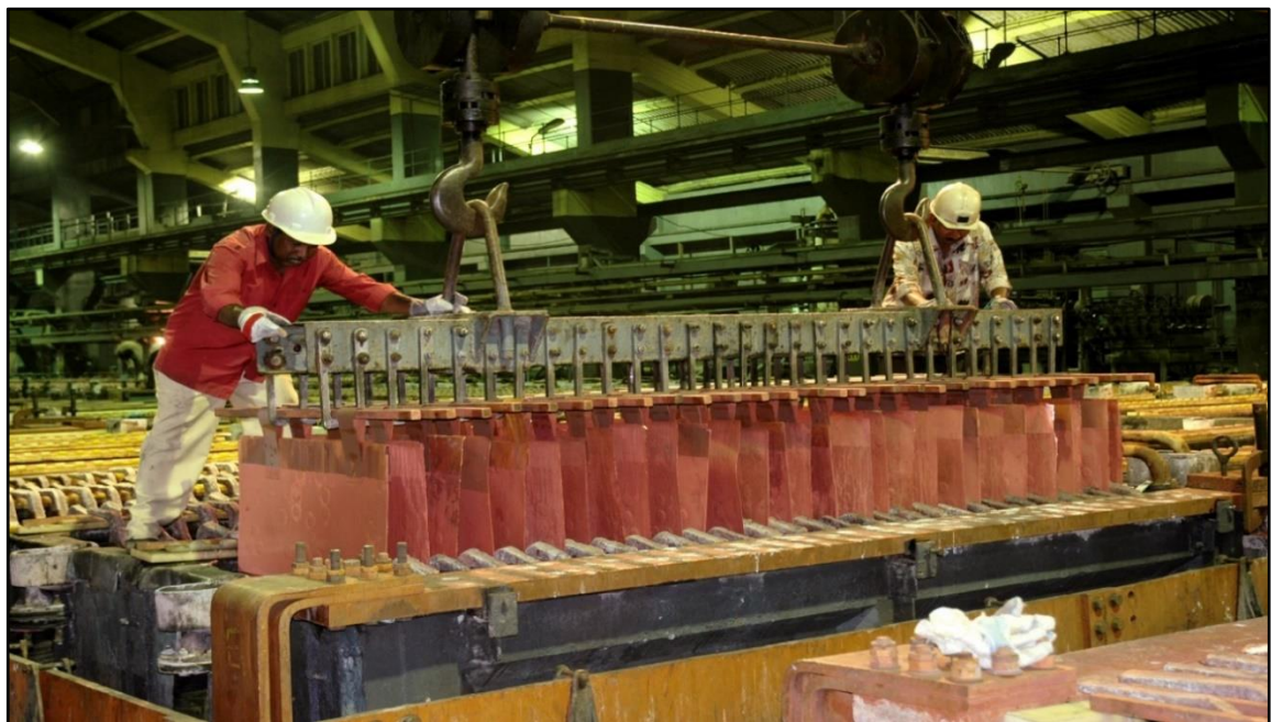
Figure: 4.3 Lifting of copper cathodes in Refinery
