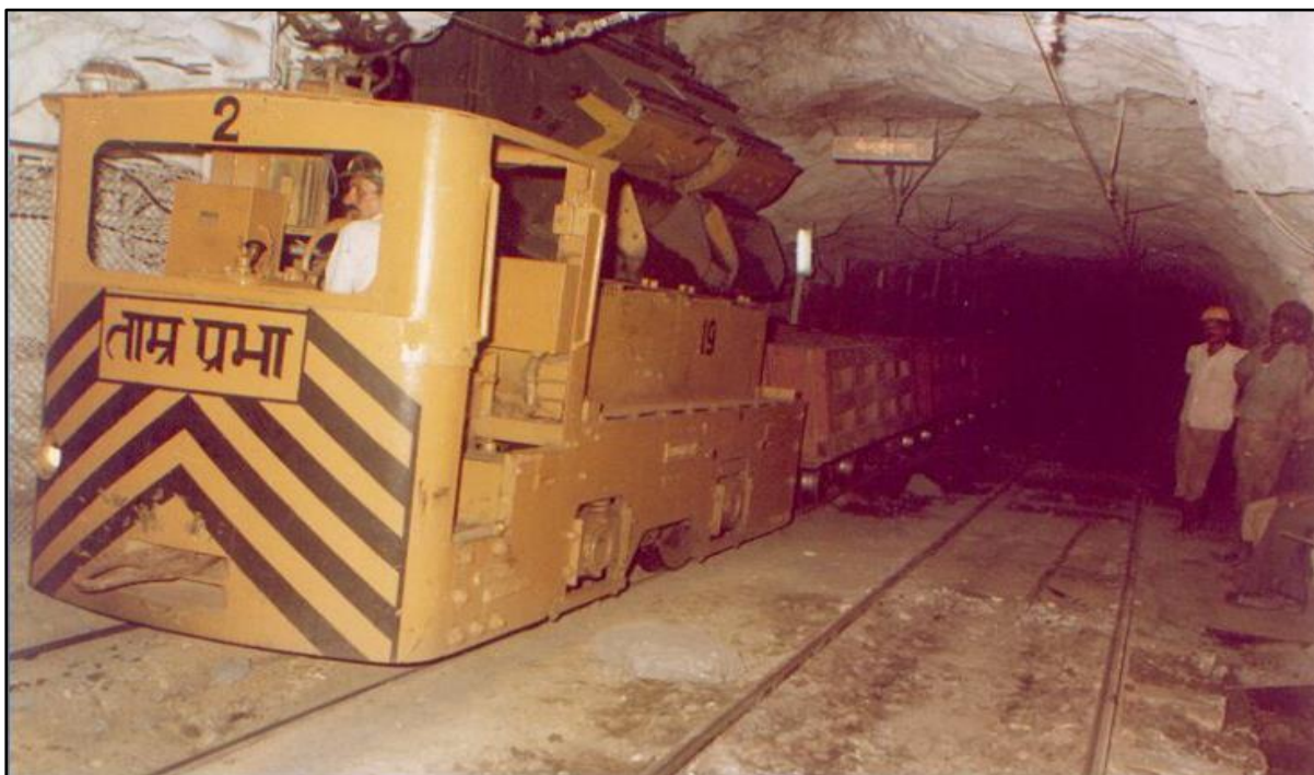
Figure 2.4: Loading of mined ores at Kolihan
