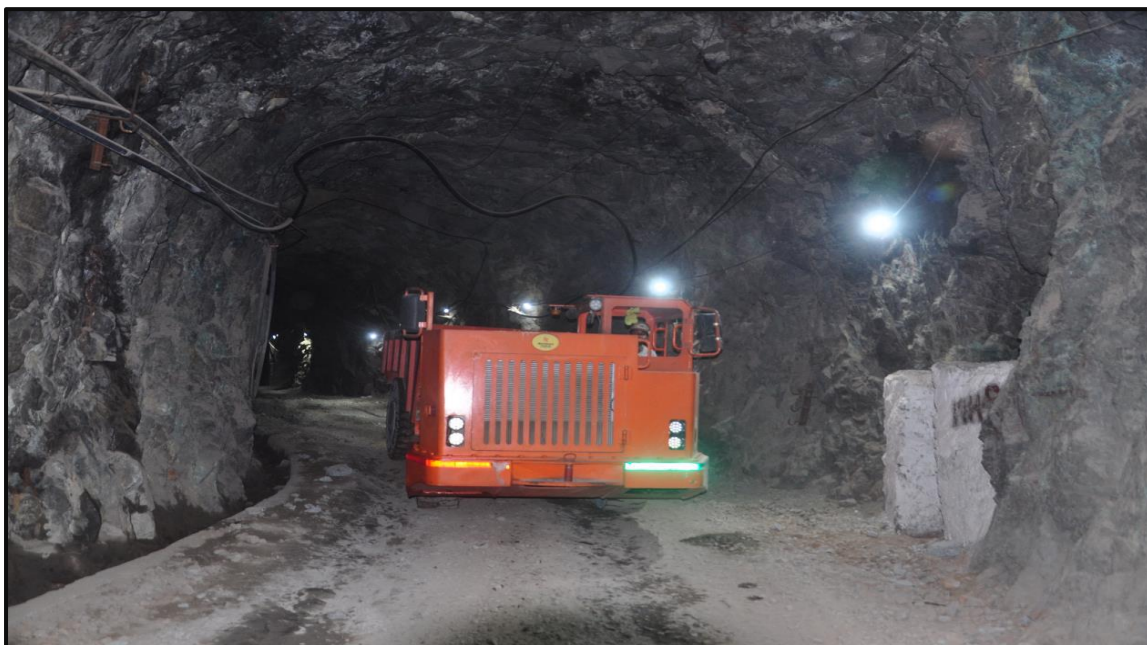
Figure 3.3: Low Profile Dump Truck operating in Malanjkhanda underground mines
