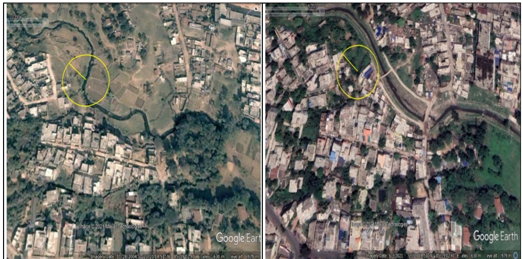
Picture 4.14: Satellite images of the river (Geographical co-ordinates: 23°21'14.51''N and 85° 19' 2.41'' E), showing encroachment of land (approximately 1,844 sq metres) The meandering flow of the river, prior to its rejuvenation (date of image: 28 November 2004) The meandering portion was straightened after rejuvenation of the river (date of image: 3 June 2021)
