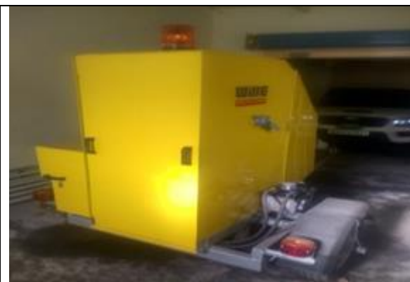
Picture No. 2.3.1: FWD equipment costing ₹ 0.55 crore (excluding vehicle cost) damaged due to keeping it exposed to harsh weather at QC Sub-Division, Bengaluru (4 th August 2021)
