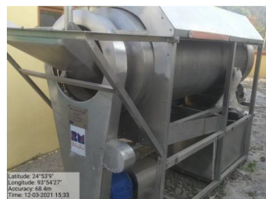
Vegetable washer lying outside without protective measure
