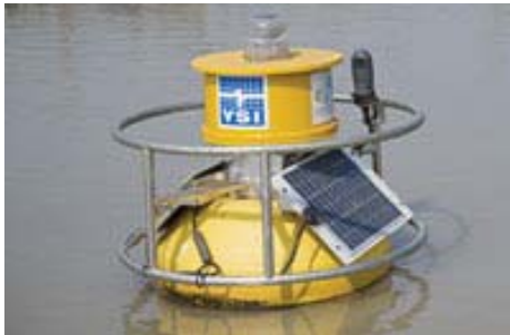
Fig. 31: Water Quality Monitoring Buoy System
