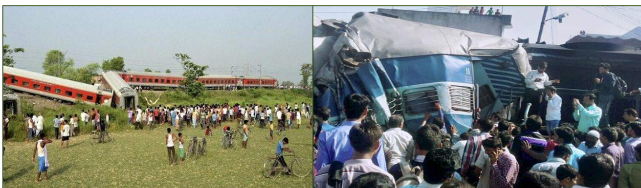
Figure 2.2: Accident site of Dibrugarh Rajdhani on 25.06.2014 - None of the LHB coaches turned turtle despite a high speed derailment and there was no loss of life (left). Accident site of Dehradun-Varanasi Janta Express near Bachrawan Railway Station on 20.03.2015 - Derailment of ICF rake claimed lives of 38 people with injury of 150 others (right).
