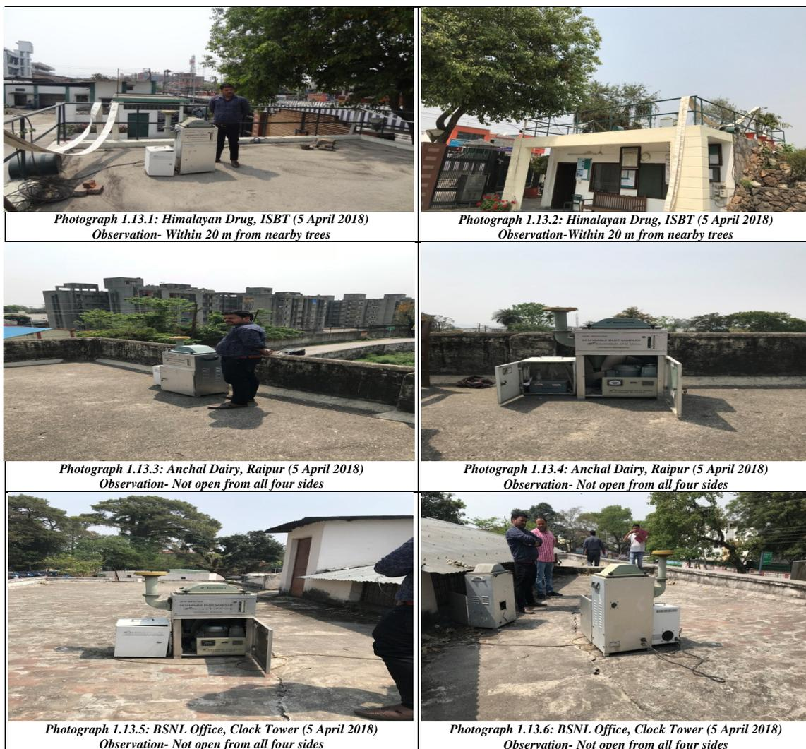
Installation of the air monitoring instruments in contravention to the prescribed norms has the risk of generating inaccurate and non-representative result.
