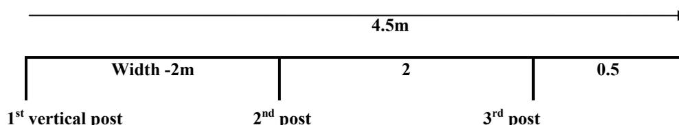
**Figure B: Requirement of vertical posts for 18 m long crash barrier as per rate analysis**
