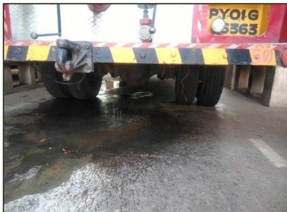
Picture 3 : Intense water leakage, Karaikal fire engine
