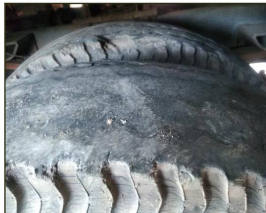
Picture 4 : Poor tyre condition, Bahour fire engine
