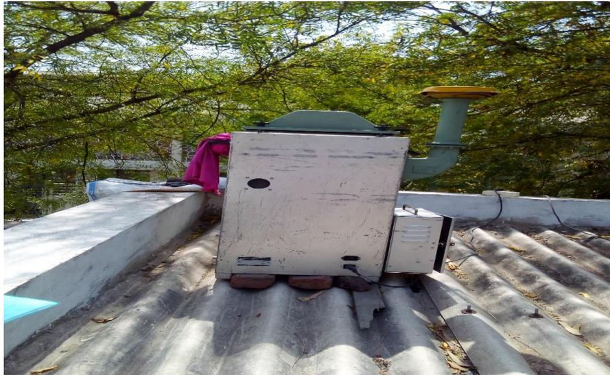
Sampler was installed at corner of roof at M/s Jain Irrigation Limited, Alwar in place of approved location and surrounded by trees which was in contravention of NAMP guidelines
