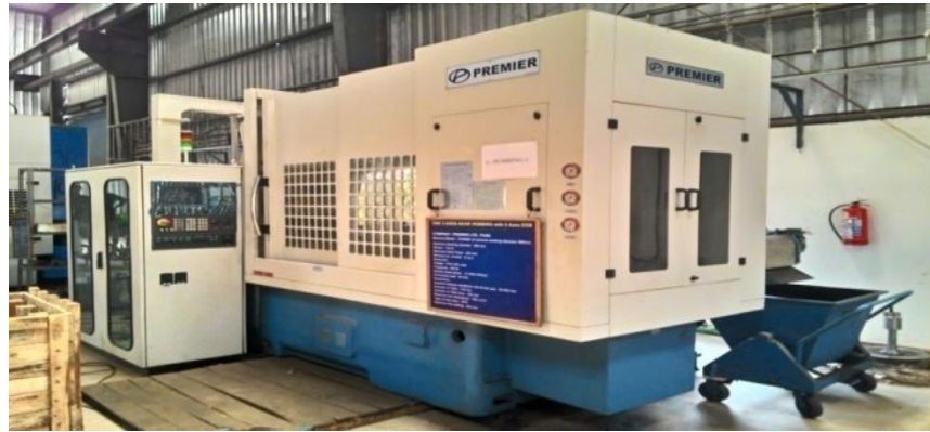
Gear hobbing machine lying idle at Machining Unit of SIFL at Shoranur
