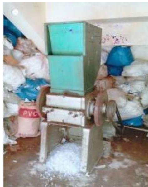
Plastic shredding machine installed at Balussery GP
