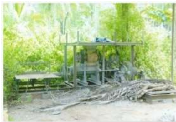
Pugmill and cutting table in the brick manufacturing unit.
