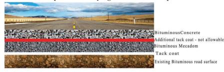
BM- a single course of 50mm thickness of compacted crushed granite premix with bituminous binder to serve as base course
