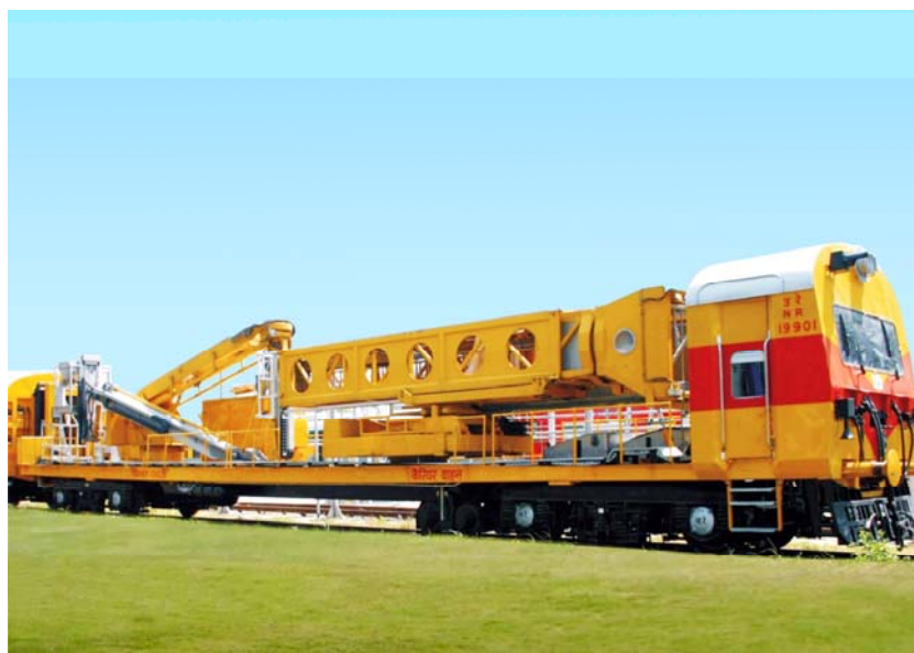
Mobile Bridge Inspection Unit manufactured at RCF, Kapurthala
