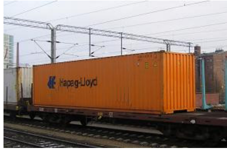
40' container loaded on a flat wagon
