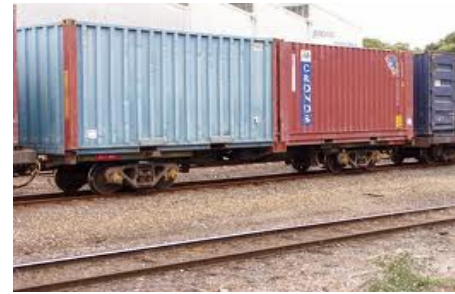
Two 20' containers loaded on a flat wagon
