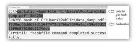
Fig. An illustration for generation of a SHA256 hash value of a (.pdf) file using command prompt.
