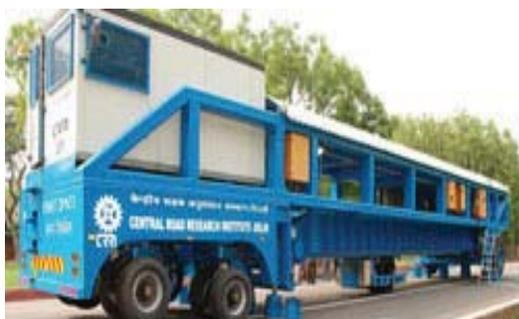
Accelerated Pavement Test Facility
