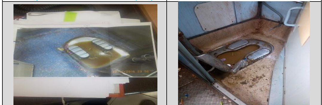
Fig 8: Choked bio-toilet in Train No 22443/44 (NCR)
